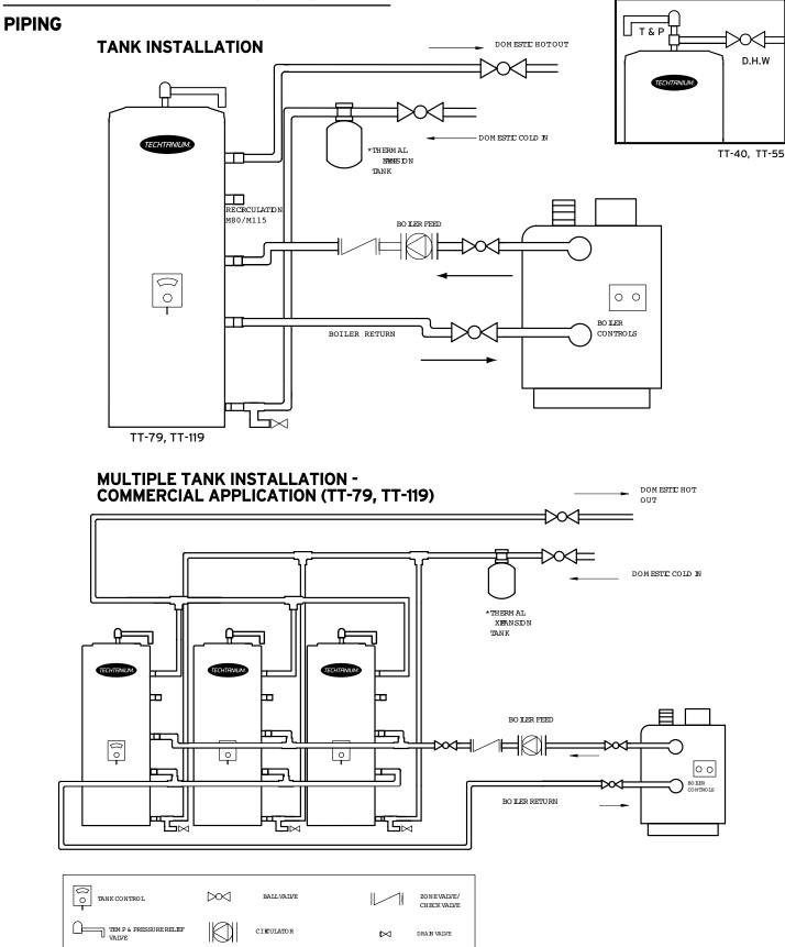
Note: Thermal Expansion Tank is required whenever a backflow preventer or no return valve is present in the system. Locate the Thermal Expansion Tank on the Domestic Cold water line between the heater and backflow preventer or no return valve.
