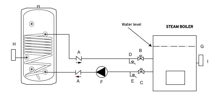
NOTE: When installing the Techtanium Indirect Water Heater with a steam boiler, the water flow (direction) is reversed through the tank coil (heat exchanger). The boiler water enters at the bottom of the coil and exits from the top of the coil. At no time should live steam be used in the tank coil (heat exchanger).
