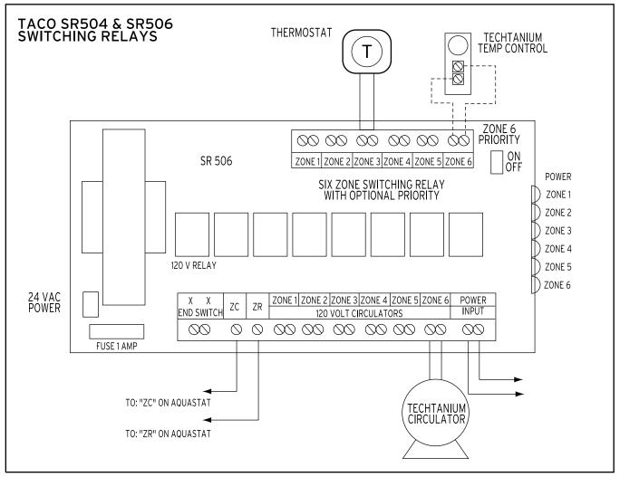
**Operation:** When any thermostat calls for heat, the boiler is given a signal to start. The appropriate circulator is energized only when the boiler temperature is above the set low limit.
