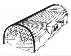
Installation or removal direct through heavy steel coil boxes welded in at any desired point along right or left sides of the boiler. It requires clearance equal to the width of the boiler measured at the top of the tubes.
