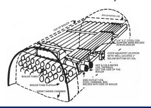
Installation and removal through front steel "Coverall" plate but with cast bronze terminals out right or left side of the boiler through welded-in-heavy steel angle terminal boxes. Fits all steel boilers where coil and piping would otherwise have to be installed through the front or rear smoke chambers.
