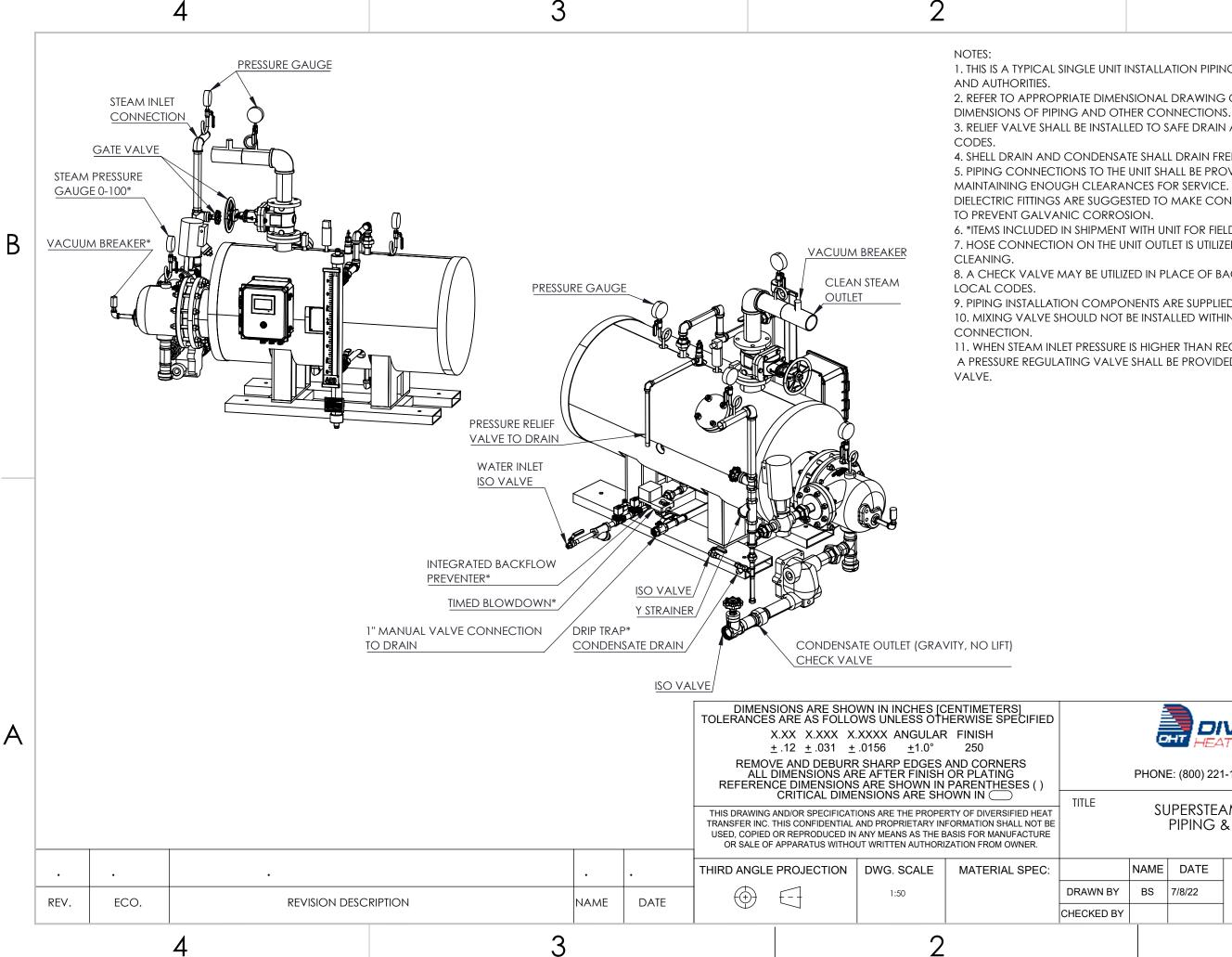
1. THIS IS A TYPICAL SINGLE UNIT INSTALLATION PIPING DRAWING. CONSULT LOCAL CODES
