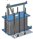
Lift the heat exchanger off the timber beams.
