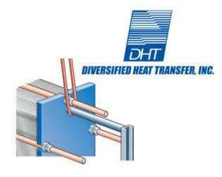
Straps should be used when lifting. Place straps according to picture.
