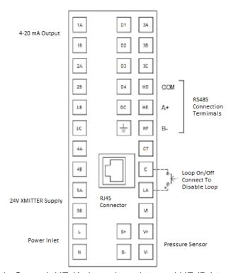
Where HD is Ground, HE (A+) receives data and HF (B-) transmits data
